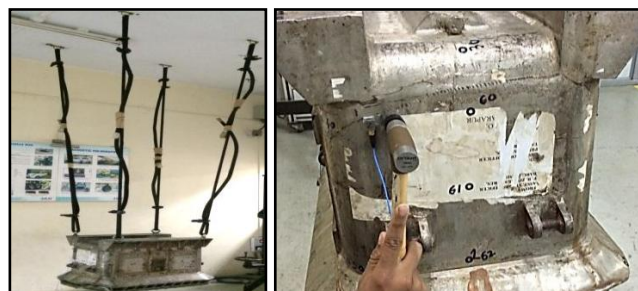
Fig. 2: Test Setup for container.
