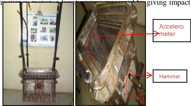
Fig. 4: Test setup for component without Lid
